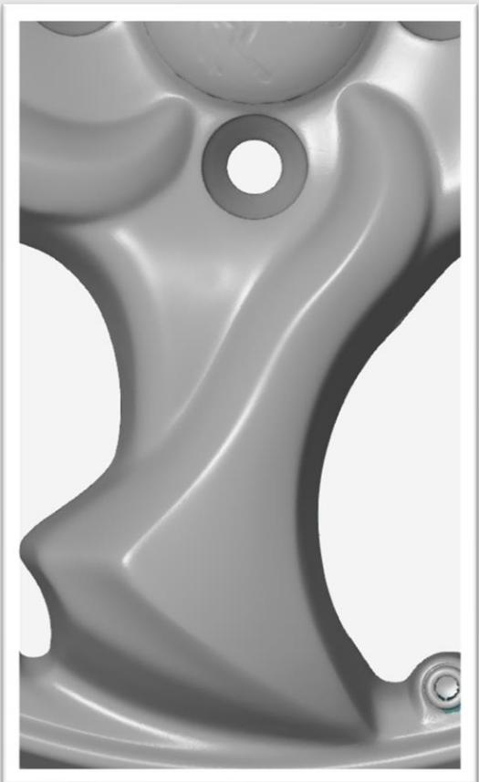
Proceed accordingly with all other sections until the entire object is digitized. Clean sprayed-over points if necessary, in order to achieve a problem-free connection of the sections.
