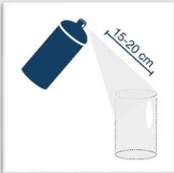
Apply AESUB blue from 15-20 cm away. Gently push down the spray button and move the can across the area using even, back and forth strokes. Move at a consistent pace to achieve an even coating. Spray over the entire surface that you will be scanning.
